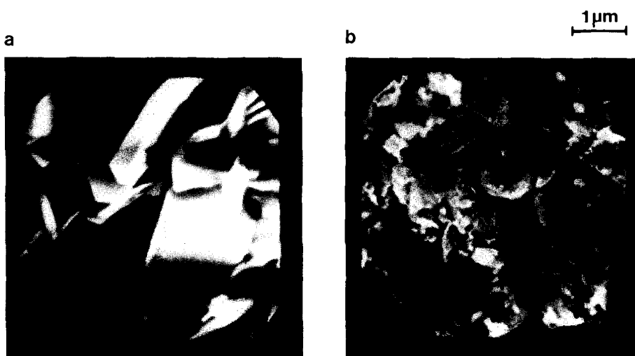
FIG. 1. SEM photographs of the U-Ni precursor (a) and the leached air-exposed U-Ni-A (b) powders.
